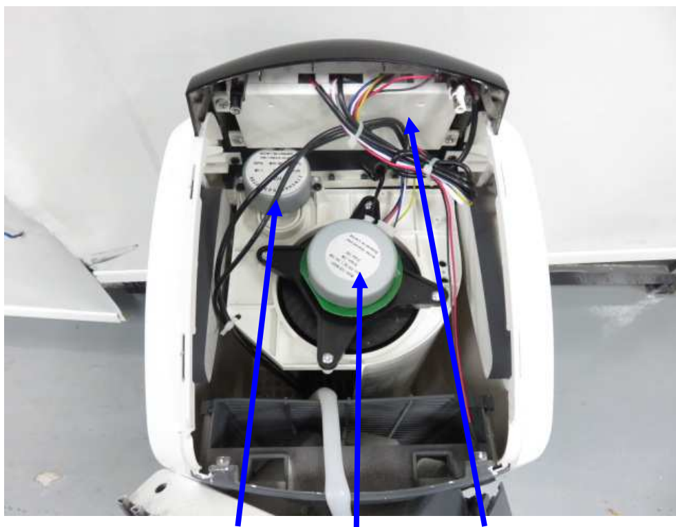
Inner view (sync. Motor, DC fan motor and main board location)
