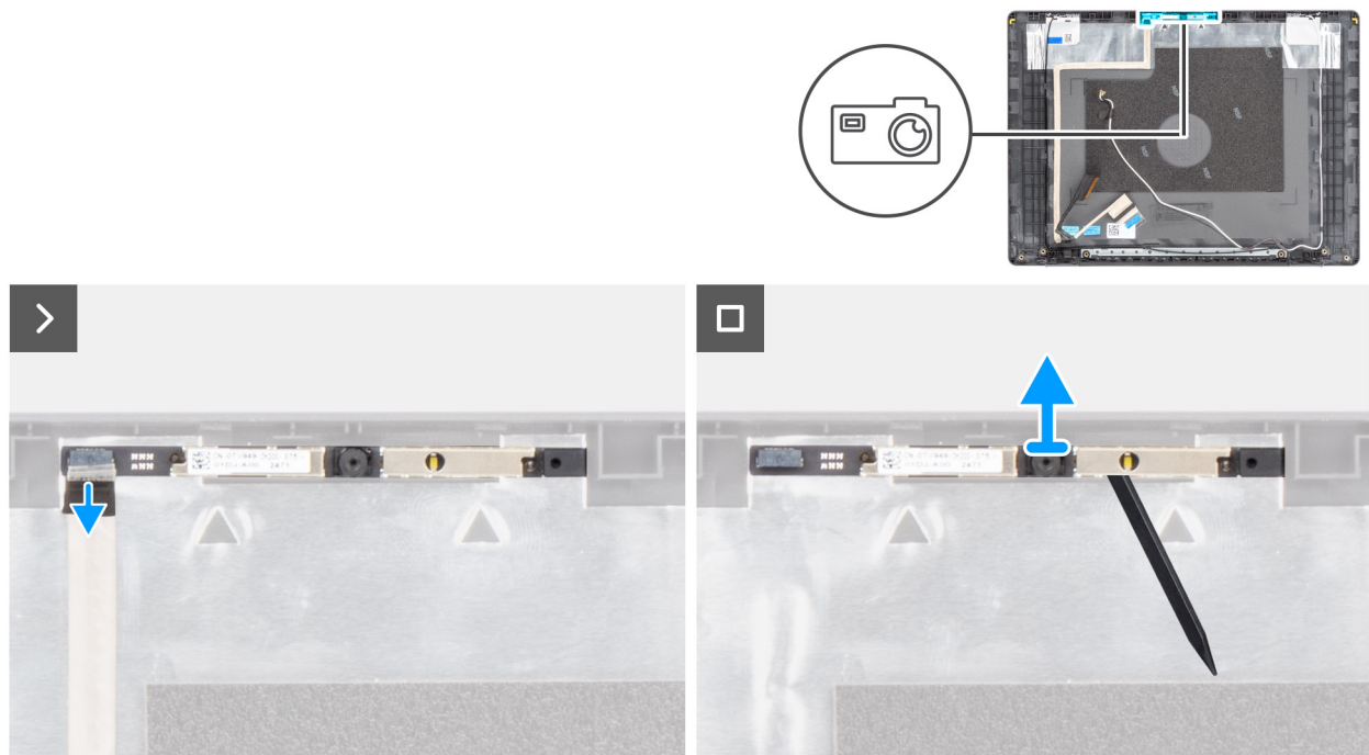
Figure 74. Removing the camera
