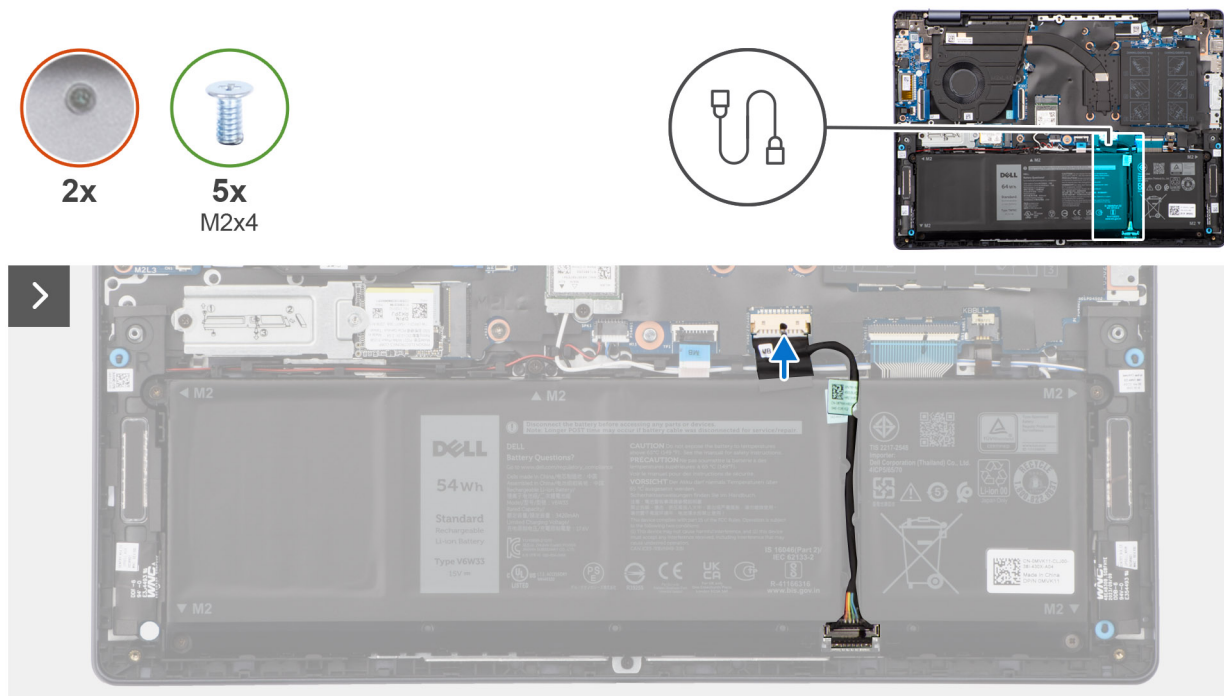
Figure 12. Connecting the battery cable
