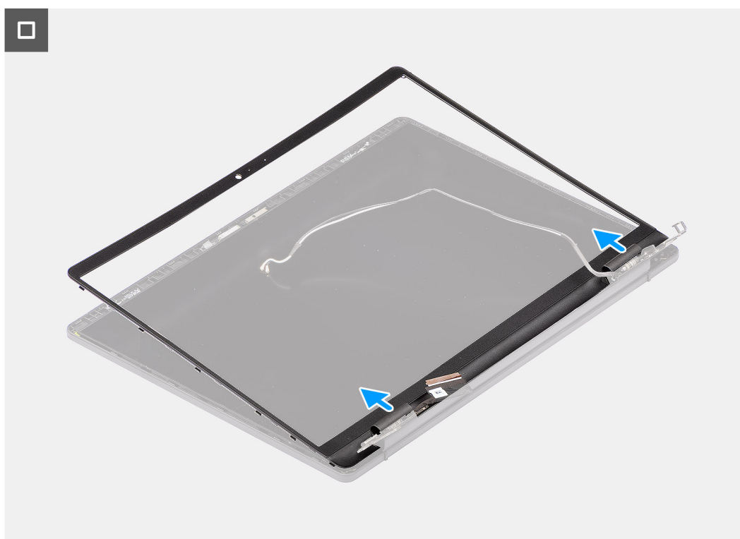
Figure 59. Removing the display bezel
