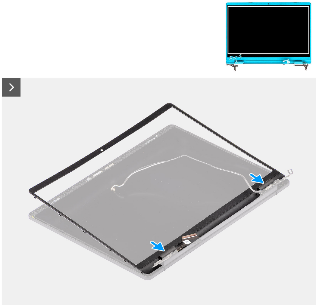
Figure 61. Installing the display bezel
