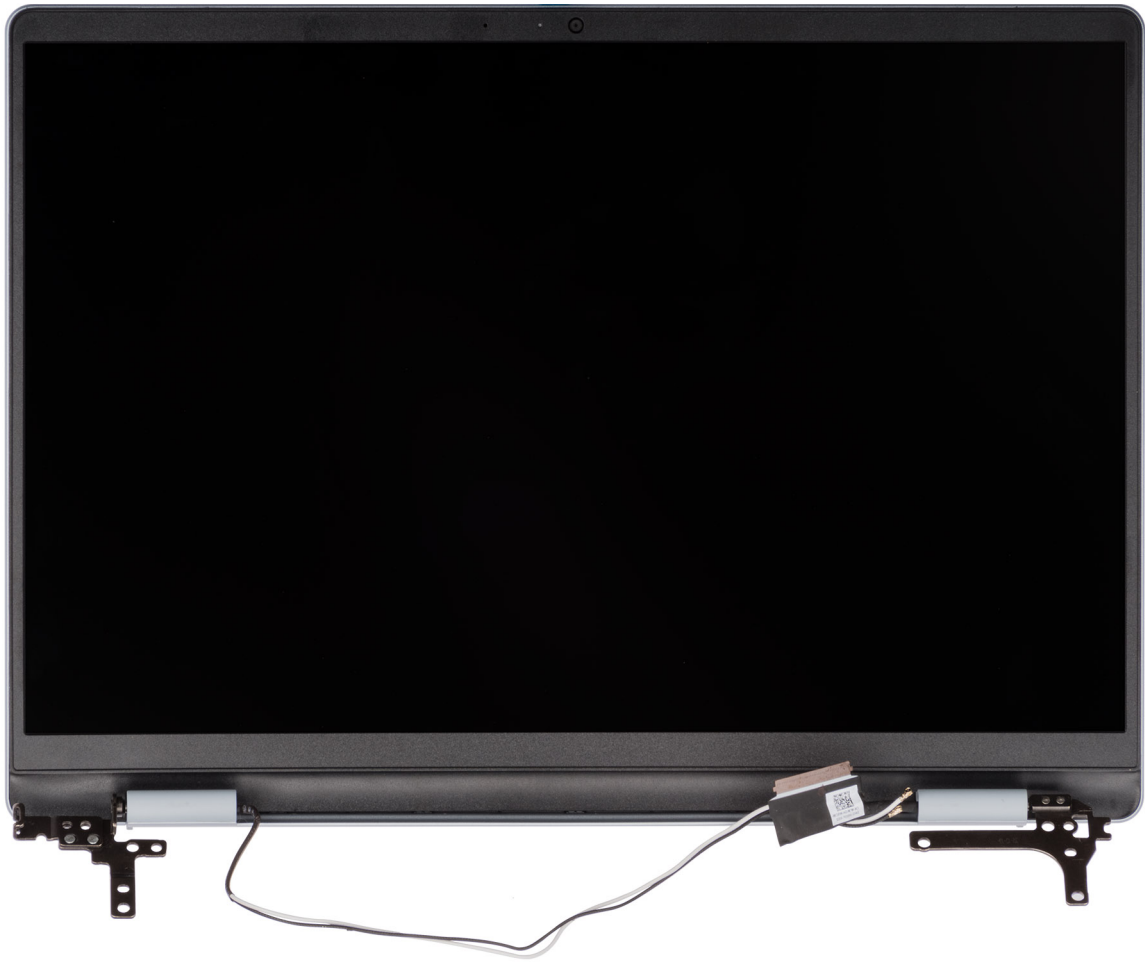
Figure 53. Display assembly (for computers shipped with a plastic chassis)
